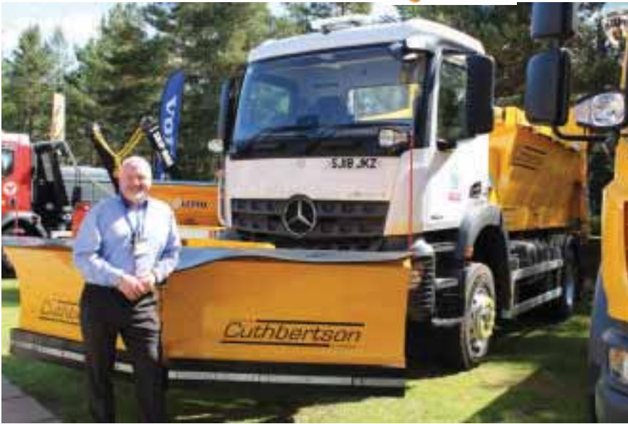
A medium duty straight V snowplough is just one of the many add-ons fitted to this Mercedes-Benz Arocs 18 tonne 4x4. As Raymond Reid (pictured) explained, it also has a multi-purpose, light weight, aluminium insulated body complete with Keith walking floor which works in both directions, hence the cantilever tailgate to allow rear loading. In addition, there's a heat resistant conveyor belt for nearside unloading and a removable grit spinner which revolves at road speed. Raymond confirmed that 13 such units are already working for Highland Council. The one on show was destined for Moray Council and another, similar Arocs is working in the colours of current Scottish Local Authority Fleet Operator of the Year, Aberdeenshire Council.
