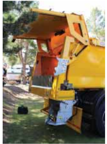
A medium duty straight V snowplough is just one of the many add-ons fitted to this Mercedes-Benz Arocs 18 tonne 4x4. As Raymond Reid (pictured) explained, it also has a multi-purpose, light weight, aluminium insulated body complete with Keith walking floor which works in both directions, hence the cantilever tailgate to allow rear loading. In addition, there's a heat resistant conveyor belt for nearside unloading and a removable grit spinner which revolves at road speed. Raymond confirmed that 13 such units are already working for Highland Council. The one on show was destined for Moray Council and another, similar Arocs is working in the colours of current Scottish Local Authority Fleet Operator of the Year, Aberdeenshire Council.
